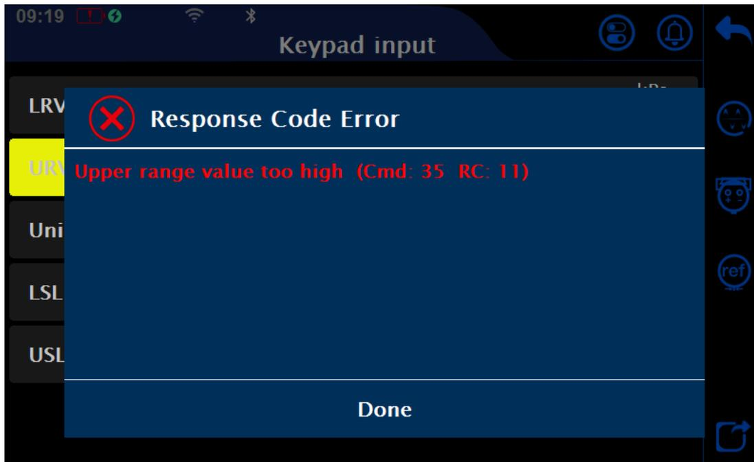
Figure 4 - Error Prompt for Sending Parameters Failure
